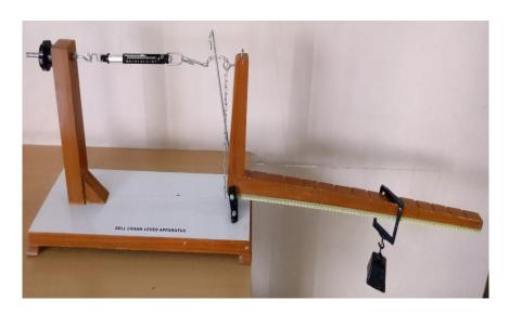
Apparatus consists of a wooden right angled lever with fulcrum at the angle, the horizontal arm is of 75cm and vertical arm is of 20cm. A spring balance with adjustable wing nut is attached to the shorter arm. The lever arm with scale is engraved at every 5cm. Apparatus is supplied with one sliding weight of 1 kg.
